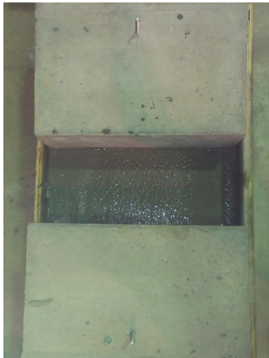
Figure 31. Push-out test specimen after overlay concrete placement
