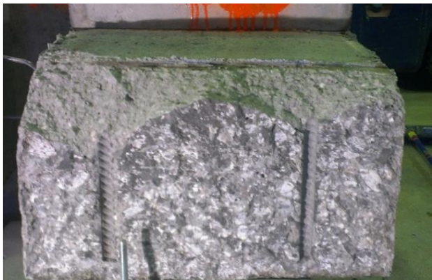
d) Bond interface (overlay concrete)
