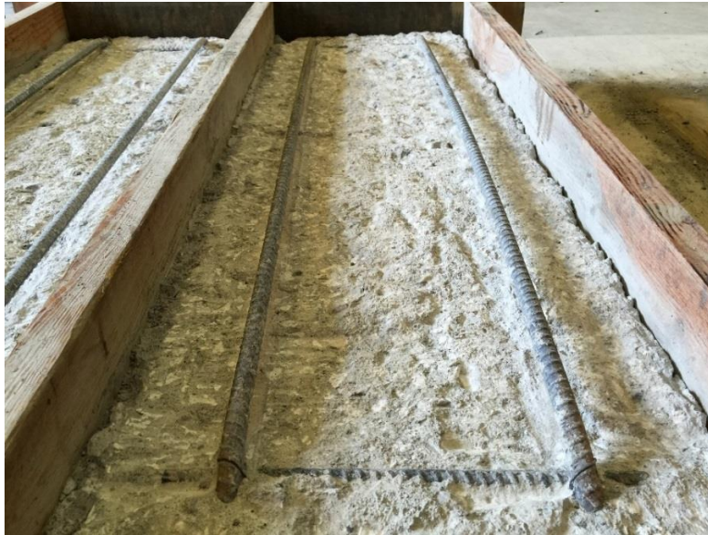
Figure 57. Negative bending flexural test specimen after concrete removal to required depth (Case 3)
