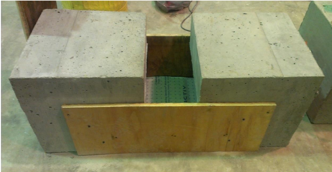
Figure 29. Push-out test formwork for overlay concrete placement
