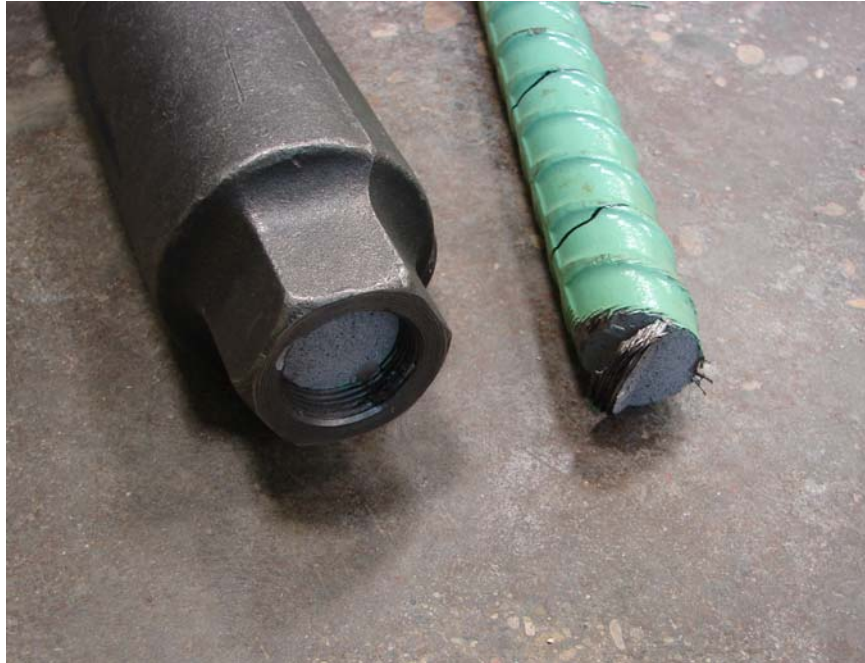
Figure 4.22 Bar fracture at threads of specimen 11AI
