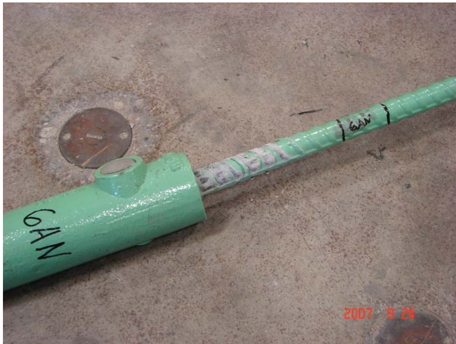
Figure 5.20 Pull-out failure of specimen 6AN
