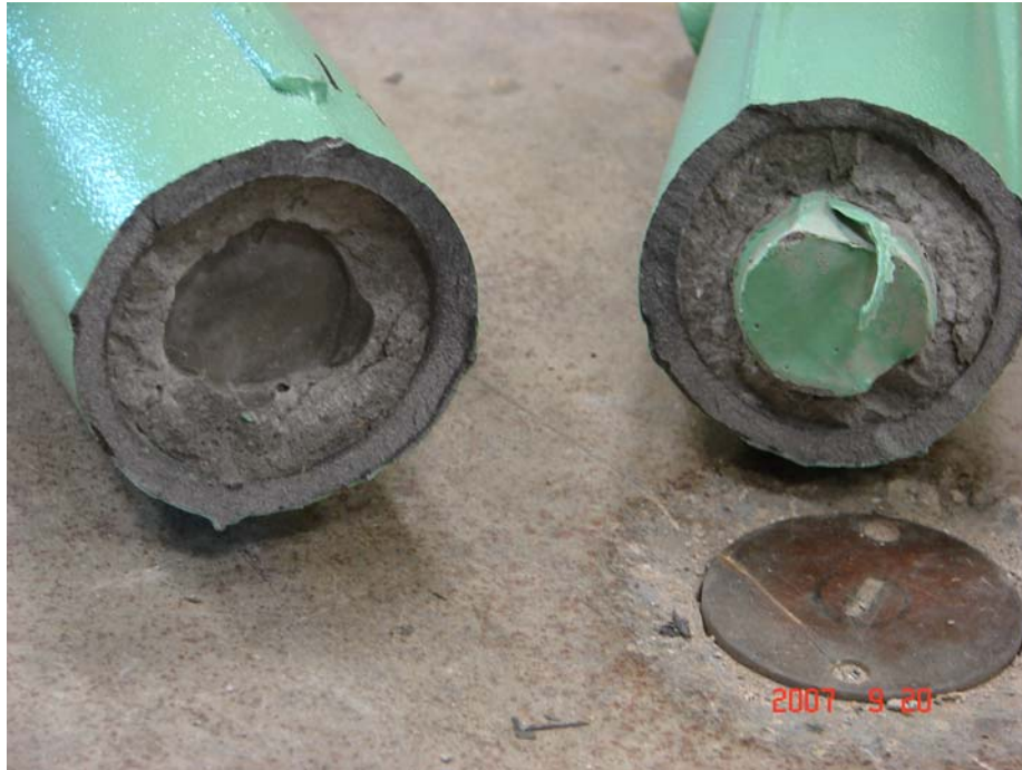
Figure 5.24 Splice fracture of specimen 11BN
