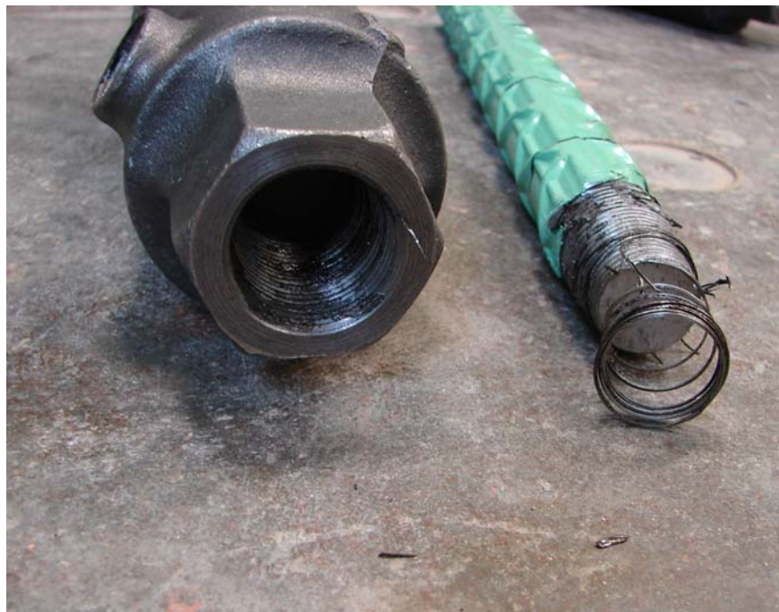
Figure 4.23 Thread failure of specimen 11BI
