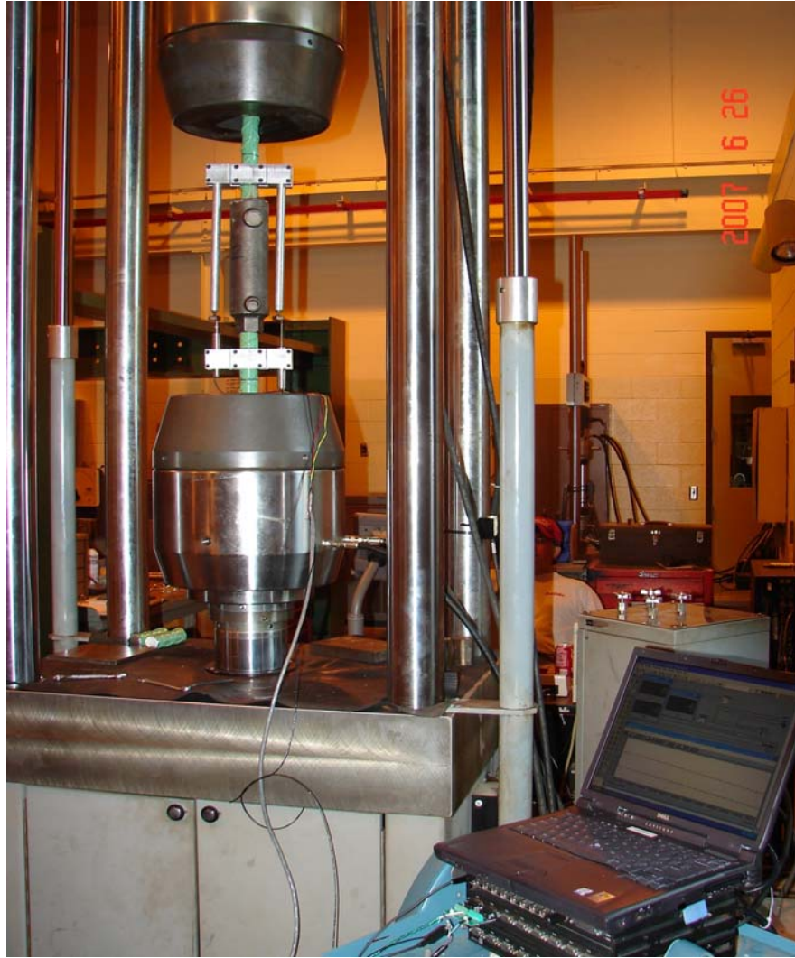
Figure 3.9 Slip test with data acquisition set up for #11 Lenton Interlok
