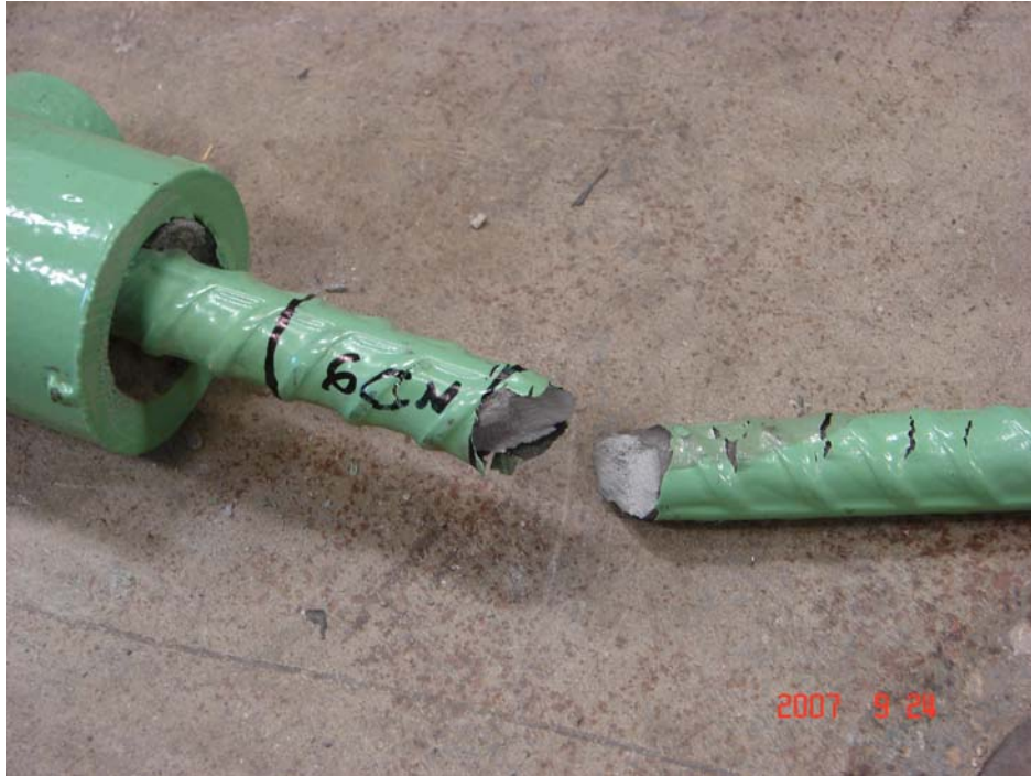
Figure 5.22 Bar fracture of specimen 6CN
