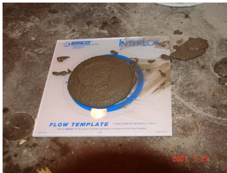
Figure 3.2 Flow template for Erico HY10L Grout
