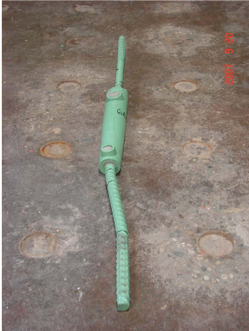
Figure 5.13 Specimen 6AN after buckling
