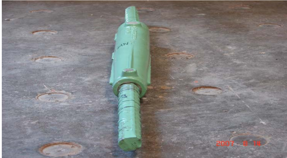
Figure 5.1 Specimen 11AN after 65 kip compressive load
