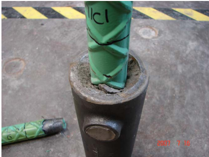
Figure 4.25 Spalling of specimen 11CI (typical of 11AI and 11BI)
