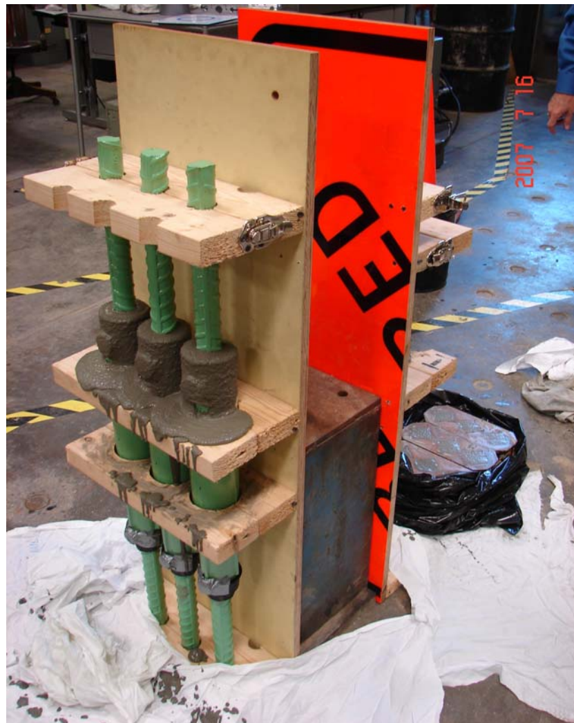
Figure 3.7 Cast #11 NMB splices
