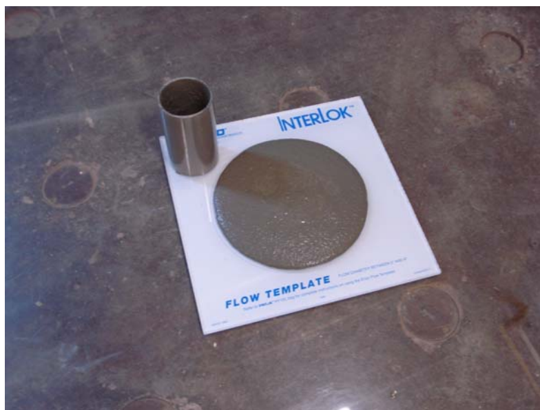
Figure 3.3 Flow template for Nissco SS Mortar
