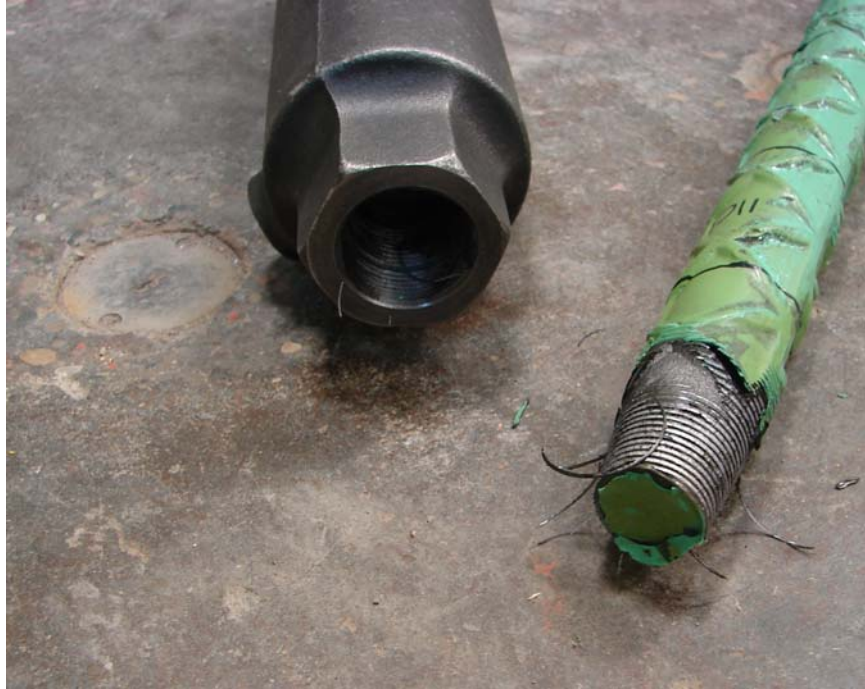
Figure 4.24 Thread failure of specimen 11CI
