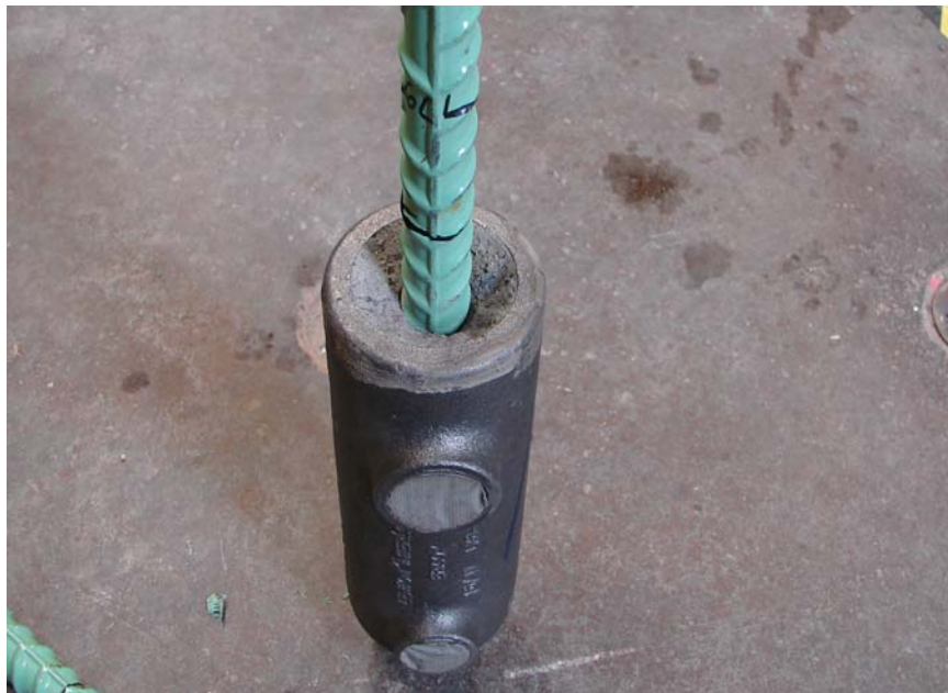
Figure 4.21 Spalling of specimen 6CI (typical of 6AI and 6BI)
