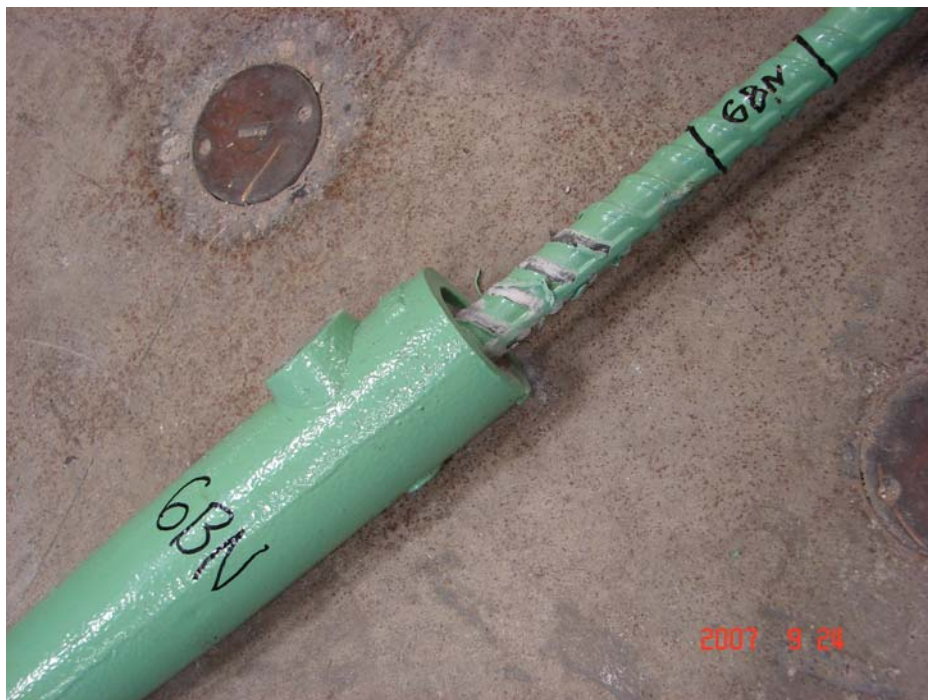
Figure 5.21 Pull-out failure of specimen 6BN
