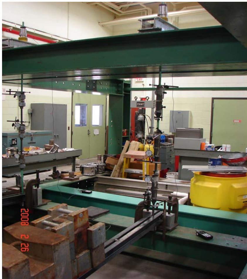
Figure 6.1 Creep test set-up
