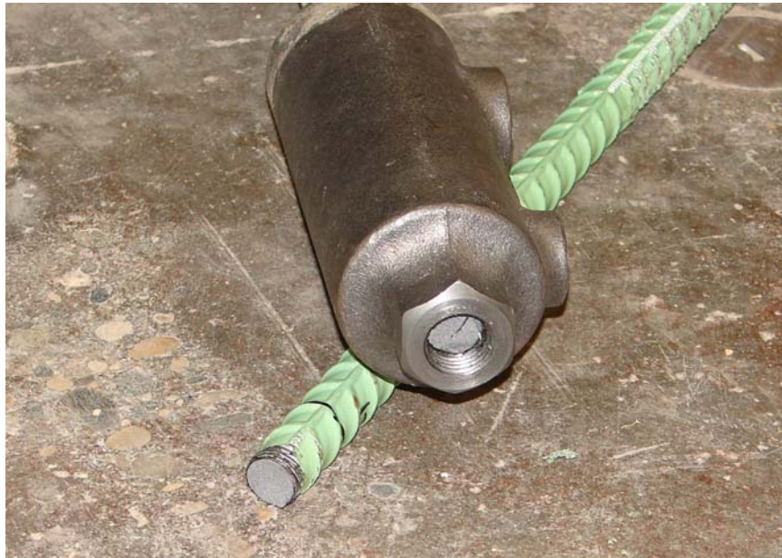
Figure 4.20 Bar fracture of specimen 6CI
