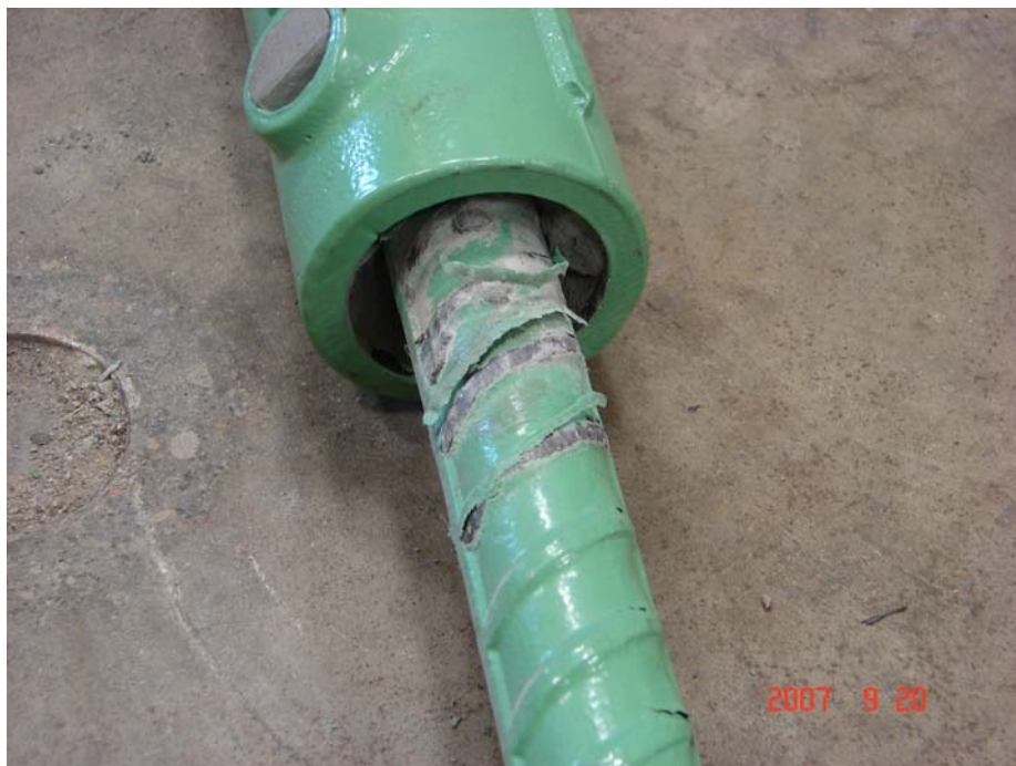
Figure 5.23 Pull-out failure of specimen 11AN
