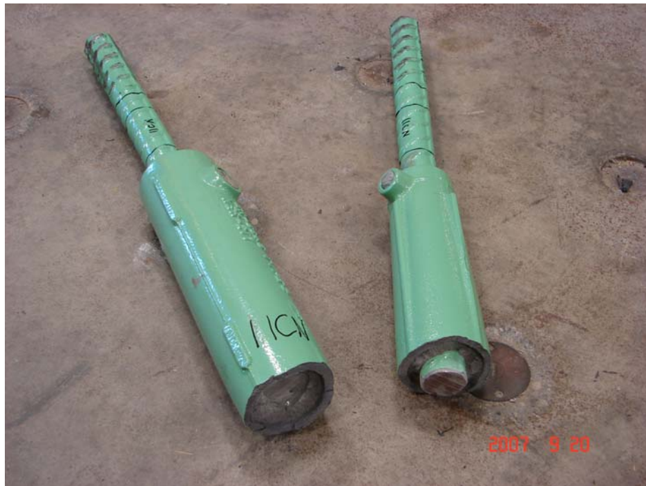
Figure 5.25 Splice fracture of specimen 11CN
