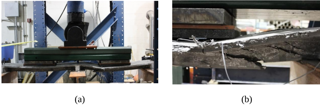
Figure 3.16 Failure Mode of Specimen 1T2S: (a) Deflected Shape, and (b) Shear Crack
